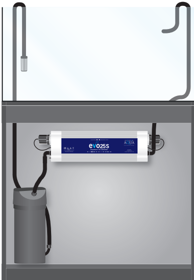
evoUV connected to external filter Fit evoUV to outlet return hose to aquarium.
