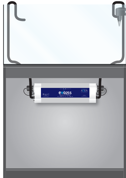
evoUV on a closed loop system Fit evoUV to a hose from pump or powerhead.
