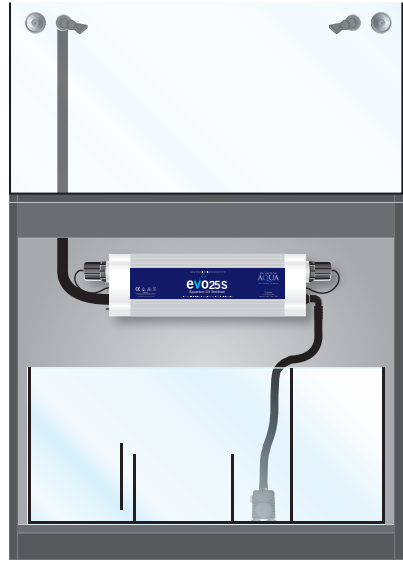
evoUV connected to pump in sump Fit evoUV to pump return to main aquarium using flexi pipe.
