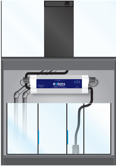
evoUV connected to pump in sump Fit evoUV to pump return to main aquarium using hard pipe.
