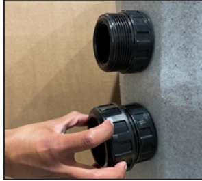
Unscrew collar from filter inlet.
